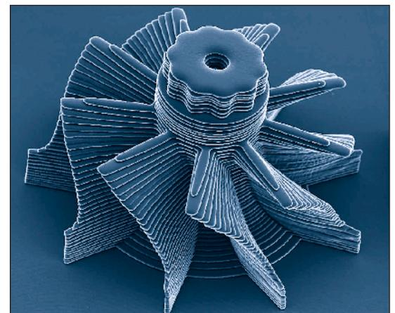
SEM (Scanning Electron Microscope) image of 1 micro-turbine part.
