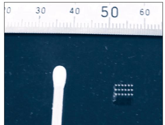
The 18 dots on the object next to the matchstick are parts built with ACCULAS : each dot is a micro-turbine of 400 microns  $\phi$  and 250 microns H - slice pitch of 5 microns.
